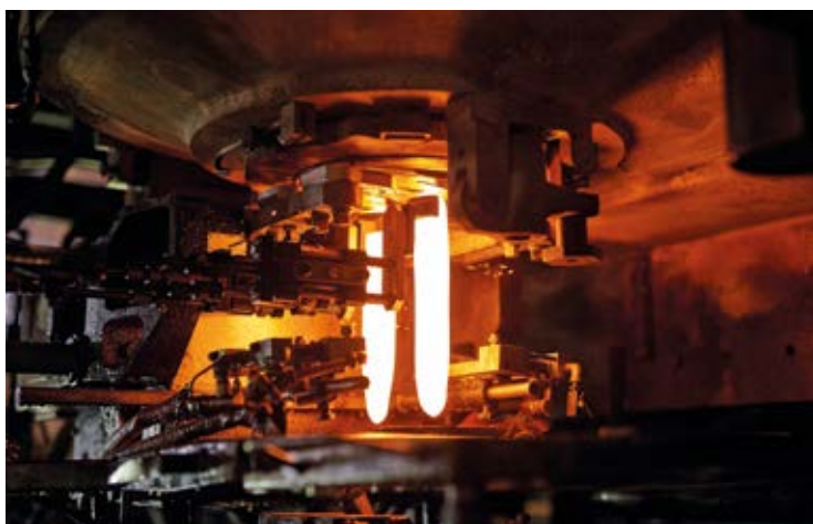
→ Parsons of melted glass © Saverglass
