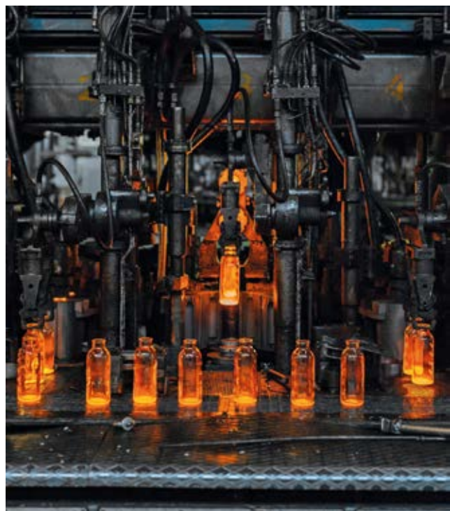
→ Individual-section (IS) machine © Shutterstock, Anton Kurashenko
