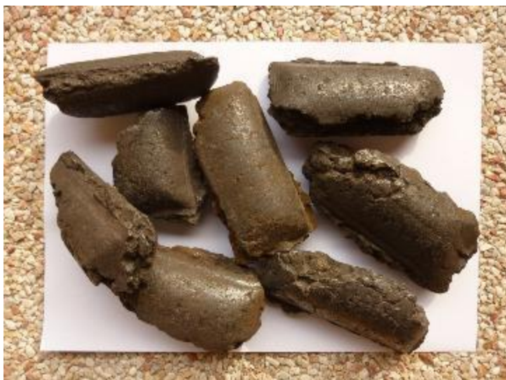
Figure 60: Direct reduced iron in the form of hot-briquettes iron, or HBI 38 .
