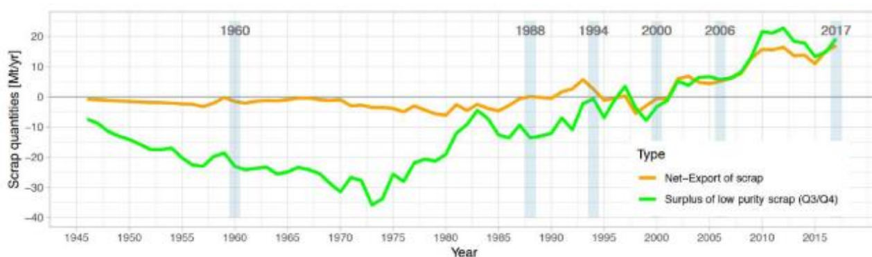
Figure24: Estimated surplus of Q3 and Q4 quality scrap and net exports of scrap from the European Union [16]
