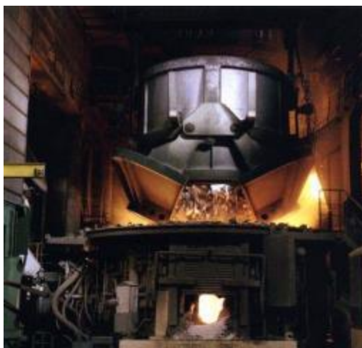
Figure 51: Charging of an electric arc furnace with a scrap metal basket [21].
